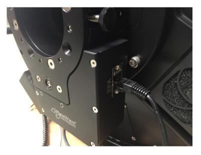
The EFA box mounted on the telescope and all cabled up. (note that in this pic, the power connector is not attached).
