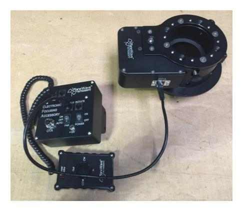
Electronics panel on the back plate of the telescope. This one is shown with the optional DeltaT dew heater option included.
